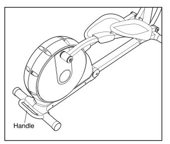
To unfold the elliptical exerciser, first hold the handle, press the latch button, and then lower the frame to the floor.
