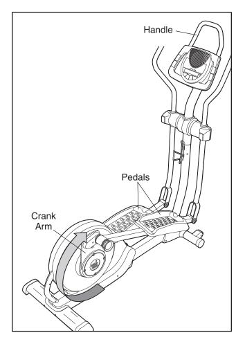
To dismount the elliptical exerciser, wait until the pedals come to a complete stop. **Note: The elliptical exerciser does not have a free wheel; the pedals will continue to move until the flywheel stops.** When the pedals are stationary, step off the highest pedal first. Then, step off the lowest pedal.
