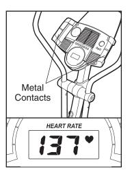
handgrips too tightly; excessive movement or pressure may interfere with heart rate readings. When your pulse is detected, the heartshaped indicator in the center display will flash each time your heart beats, and your heart rate will be shown.
