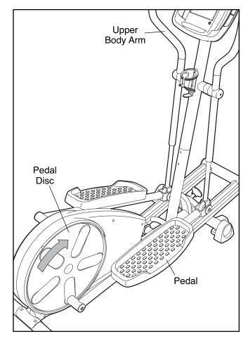
To dismount the elliptical exerciser, allow the pedals to come to a complete stop. **The elliptical exerciser does not have a freewheel; the pedals will continue to move until the flywheel stops.** When the pedals are stationary, step off the higher pedal first. Then, step off the lower pedal.
