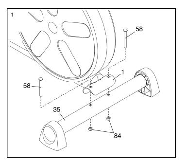
Attach the Front Stabilizer (3) to the Frame (1) with two M10 x 77mm Carriage Bolts (58) and two M10 Nylon Locknuts (84).
