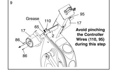
Connect the Left Handlebar Wire (108) to the Left Controller Wire (110). Insert the excess wire into the Left Handlebar (8).
