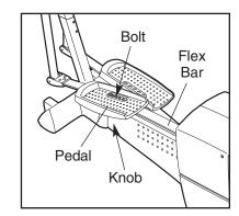
upward, slide the pedal forward or backward to the desired position, and then retighten the knob. Make sure that both pedals are in the same position.
