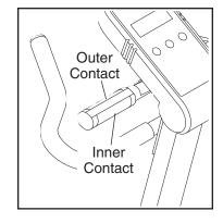
resting on the inner contacts and your fingers must be touching the outer contacts. Avoid moving your hands. When your pulse is detected, a heartshaped indicator in the display will flash. After a moment, three dashes will appear and your heart rate will be shown. For the most accurate reading, continue to hold the contacts for about 15 seconds.
