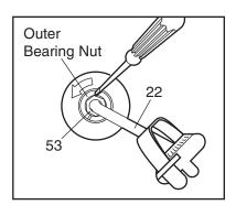
screwdriver in one of the slots in the outer bearing nut. Tap the screwdriver with a hammer to turn the outer bearing nut counterclockwise until the arms are no longer loose. **Do not overtighten the outer bearing nut.** When the outer bearing nut is properly tightened, retighten the Hex Jam Nut.
