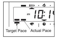
the display. The left column will show one bar, showing that the target pace is 5 mph (8 kph). The right column will show your actual pedaling pace. Adjust your pedaling pace until only one bar appears in the right column. Each time the target pace changes during the program, adjust your pedaling pace to keep both columns at the same height.
