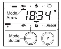
selected, the console will display the speed, time, distance, lap and calorie modes, for 5 seconds each, in a repeating cycle.
