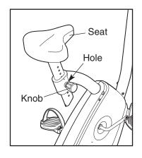
slide the seat post up or down, and align one of the adjustment holes in the seat post with the indicated hole in the seat frame. Insert the seat knob into the seat frame and the seat post, and turn the knob clockwise until it is tight. Make sure that the seat knob is inserted through one of the adjustment holes in the seat post.
