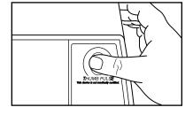
ed—fully press it down. **Do not press too hard, or** the circulation in your thumb will be restricted, and your pulse will not be detected. Next, raise your thumb slightly until the heart-shaped indicator in the right display flashes **steadily**. Hold your thumb at this
