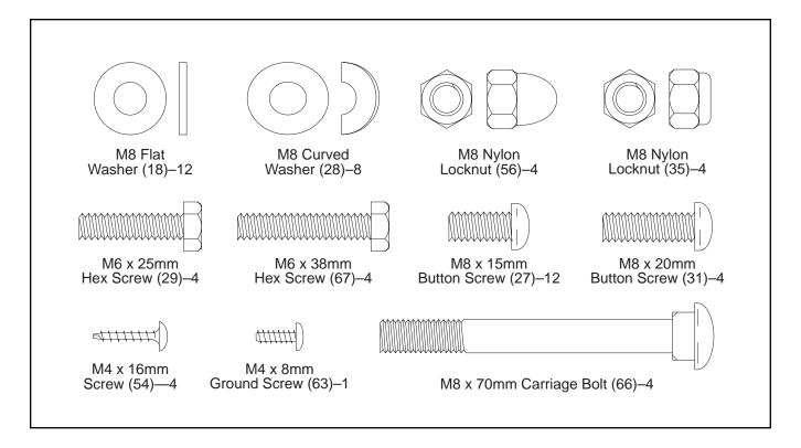
Identify the Front Stabilizer (2), which is shorter than the Rear Stabilizer (not shown). Attach the Front Stabilizer to the front of the Frame (1) with two M8 x 70mm Carriage Bolts (66), two M8 Curved Washers (28), and two M8 Acorn Nuts (56).
