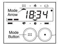
scan mode is selected, the console will display the speed, time, distance, lap and calorie modes, for 5 seconds each, in a repeating cycle.
