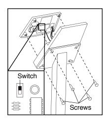
to change the unit of measurement. Reattach the console with the four screws. **Be careful not to pinch any of the wires.**
