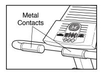
your fingers must be touching the lower contacts. **Avoid moving your hands.** After a moment, the heart-shaped indicator in the display will begin to flash and your heart rate will be shown. For the most accurate heart rate reading, continue to hold the contacts for about 15 seconds.
