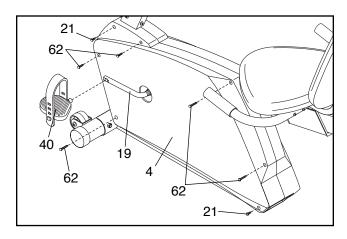
Using an adjustable wrench, turn the Left Pedal (40) clockwise and remove it from the Crank (19). Next, remove the two M4 x 16mm Screws (21) and the five M4 x 38mm Screws (62) from the Left Side Shield (4). Make sure that the left arm of the Crank is in the position shown above and carefully slide the Left Side Shield forward off the arm of the Crank.
