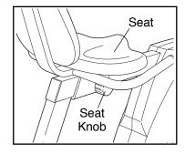
adjust the seat, make sure that your knees will not touch the handlebar or the console when you pedal. To adjust the seat, first turn the seat knob counterclockwise two or three turns to loosen it (if the seat knob is not loosened enough, it may scratch the frame). Next, pull the seat knob, slide the seat to the desired position, and then release the seat knob. Make sure to move the seat back and forth slightly until it locks in position. Then, turn the seat knob clockwise to tighten it.
