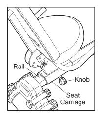
to loosen it (if the knob is not loosened enough, it may scratch the rail). Next, pull the knob, slide the seat carriage to the desired position, and then release the knob. **Move the seat carriage back and forth slightly until it locks into position.** Then, turn the knob clockwise until it s tight.
