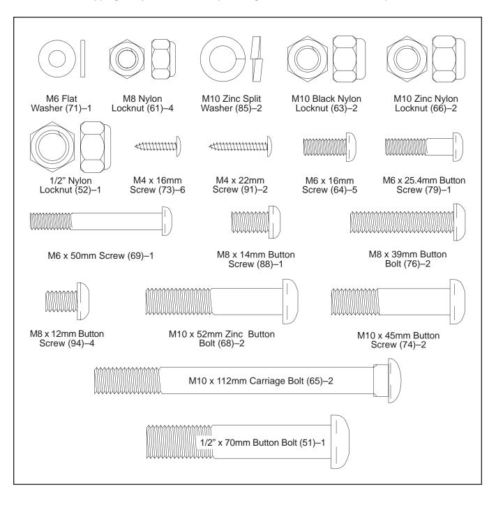
While another person lifts the front of the Frame (1), attach the Front Stabilizer (2) to the Frame with two M10 x 112mm Carriage Bolts (65) and two M10 Black Nylon Locknuts (63). Make sure that the Front Stabilizer is turned so the Wheels (30) are not touching the floor.
