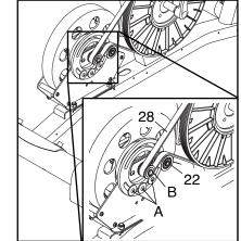
Belt (28) is tight. Then, tighten the three screws.
