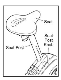
the adjustment holes in the seat post. Then, turn the knob clockwise to tighten it.
