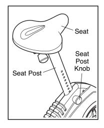
upward or downward to the desired position, and then release the knob. Move the seat post upward or downward slightly to make sure that the knob is engaged in one of the adjustment holes in the seat post. Then, turn the knob clockwise to tighten it.
