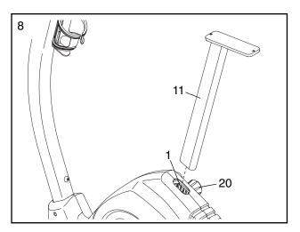
Attach an M6 x 10mm Screw (60) to the Seat Post (11). Next, slide the Seat Carriage (19) onto the Seat Post. Then, adjust the Seat Carriage to the desired position and tighten the Seat Knob (31) into the Seat Carriage.
