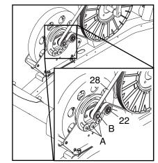
Belt (28) is tight. Then, tighten the three screws.
