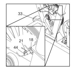
Reed Switch slightly closer to or away from the Magnet. Then, retighten the Screw. Turn the Crank for a moment. Repeat until the console displays correct feedback. When the Reed Switch is correctly adjusted, reattach the left side shield and the left pedal.
