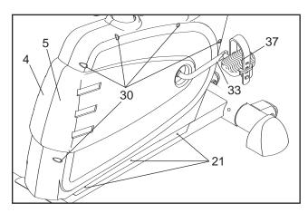
Shield. Using an adjustable wrench, turn the Right Pedal (37) counterclockwise and remove it. Next, turn the Crank (33) so that it points toward the front of the exercise cycle, and then slide off the Right Side Shield.
