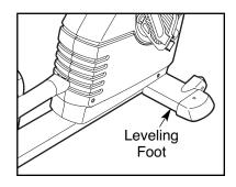
ing use, turn one or both of the leveling feet under the front stabilizers until the rocking motion is eliminated.
