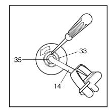
driver in one of the slots in the Slotted Bearing Nut (33). Lightly tap the screwdriver with a hammer to turn the Slotted Bearing Nut counterclockwise until the arms are no longer loose. **Do not overtighten the Slotted Bearing Nut.** When the Slotted Bearing Nut is properly tightened, tighten the Crank Nut.
