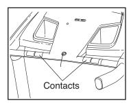
To use the handgrip pulse sensor, **stand on the foot rails** and hold the metal contacts for at least ten seconds—**avoid moving your hands**. When your pulse is detected, your heart rate will be shown. For the most accurate heart rate reading, continue to hold the contacts for about 15 seconds. 7. When you are finished exercising, remove the key from the console.
