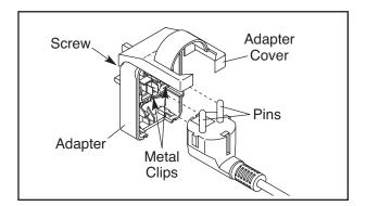
3. Plug the power cord into an appropriate outlet that is properly installed and earthed in accordance with all local codes and ordinances.
