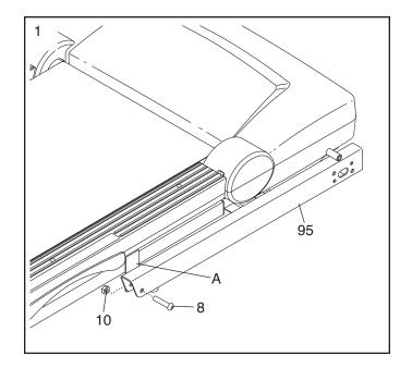
With the help of a second person, carefully tip the treadmill onto its left side. Partially fold the Frame (55) so that the treadmill is more stable; do not fully fold the Frame yet.
