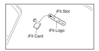
Next, select an iFit workout by pressing the iFit increase and decrease buttons next to the iFit slot. When an iFit workout is selected, the workout duration, the maximum incline setting, the name, and the maximum speed setting of the workout will appear in the displays. In addition, a profile of the speed settings of the workout will scroll across the matrix.
