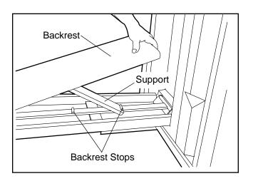
To adjust the backrest to the level position, first raise the backrest slightly. Pivot the end of the support in the direction shown by the arrow. Lower the backrest onto the bench frame.
