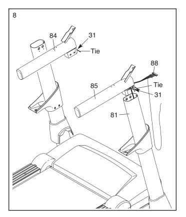
Attach the Right Handrail (85) to the Right Upright (81) with two 5/16" x 1" Bolts (5), two 5/16" Star Washers (13), and a 5/16" x 1 1/4" Bolt (2). Do not fully tighten the Bolts yet.
