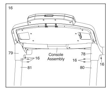
Attach the Left Tray (101) and the Right Tray (102) to the console assembly with four #8 x 1/2" Screws (16).
