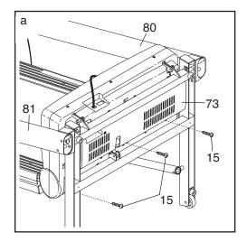
Remove the three #8 x 3/4" Screws (1) and carefully pivot the Motor Hood (61) off.
