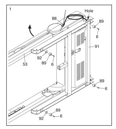
2. See the inset drawing. Cut the plastic tie near the Upright Wire (88).
