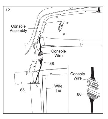
Set the console assembly on the Left Handrail (84) and the Right Handrail (85). Be careful not to pinch any wires. Insert the excess Upright Wire (not shown) into the Right Handrail.
