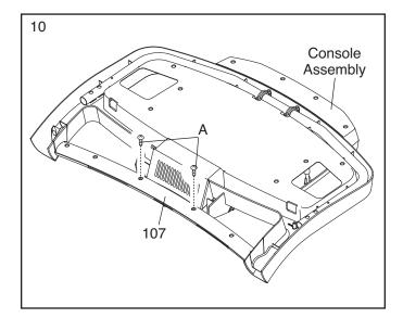
11. IMPORTANT: To avoid damaging the Crossbar (107), do not use power tools and do not overtighten the #10 x 3/4" Screws (4) or the #10 x 3/4" Flat Head Screws (109).
