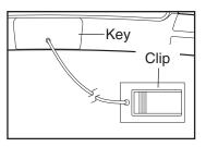
ment, the displays will light. **IMPORTANT: In an emergency, the key can be pulled from the console,** causing the walking belt to slow to a stop. Test the clip by carefully taking a few steps backward; if the key is not pulled from the console, adjust the position of the clip.
