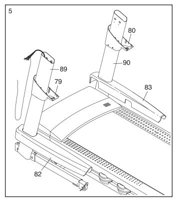
Cut the plastic tie in the Left Handrail (88) and the Right Handrail (not shown). If necessary, press the 5/16" Cage Nuts (31) back into place.
