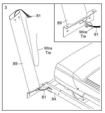
Hold the Left Upright (89) against the Base (94). Be careful not to pinch the Upright Wire (81). Insert two 3/8" x 1 1/4" Bolts (8) with two 3/8" Star Washers (13) and two 3/8" x 2 3/4" Bolts (7) into the Left Upright.
