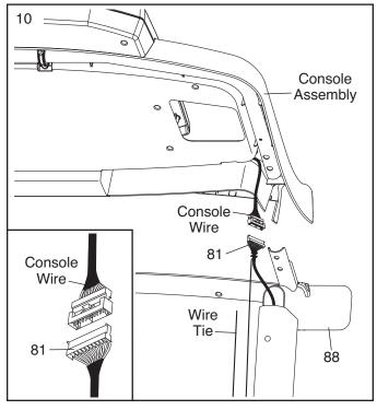
Set the console assembly on the Left Handrail (88) and the Right Handrail (87). Be careful not to pinch any wires. Insert the excess Upright Wire (not shown) into the Left Handrail.
