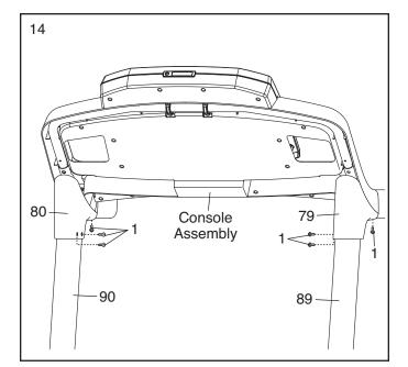
Attach the Left Tray (107) and the Right Tray (108) to the console assembly with four #8 x 1/2" Screws (1).
