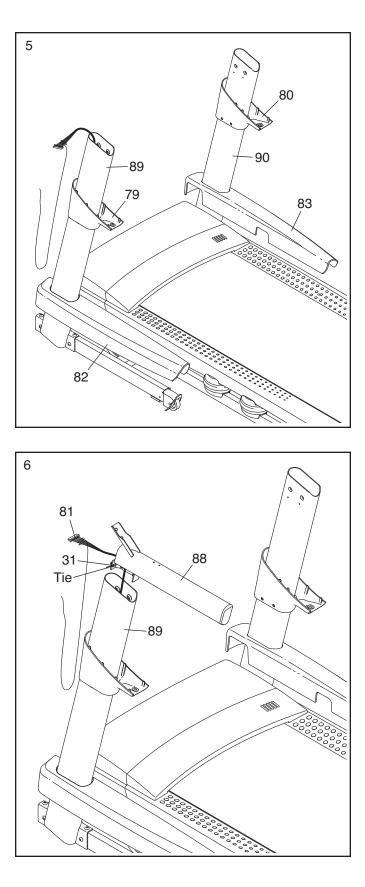
Attach the Left Handrail (88) to the Left Upright (89) with two 5/16" x 1" Screws (5), two 5/16" Star Washers (11), and a 5/16" x 1 1/4" Bolt (4).
