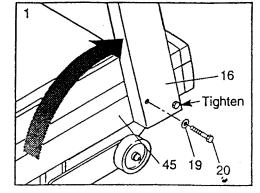
2. With the help of a second person, rotate the Handrail (7) up as shown. Insert two Handrail Lock Bolts (1) into the Left and Right Uprights (2, 16) and tighten the Bolts with the 7/32" Allen Wrench (91).
