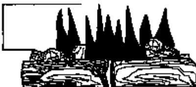
Figure 21 -Incorrect Flame Pattern with Control Knob Set to High Flame
