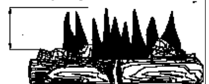
Figure 16 - Incorrect Flame Pattern With Control Knob Set to High Flame
