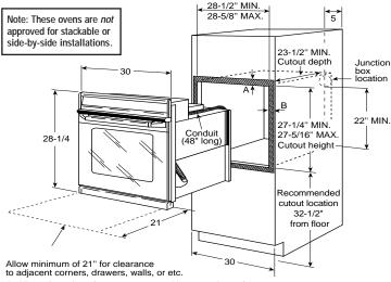
A=Allow 1" overlap of oven over top and bottom edges of cutout. B=Allow 11/16"-3/4" for overlap of oven over side edges of cutout.
