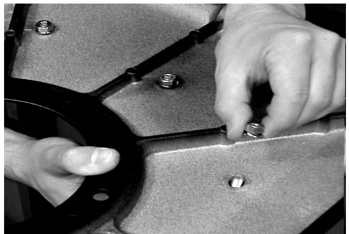
Figure 3 Attaching Pedestal to Base
