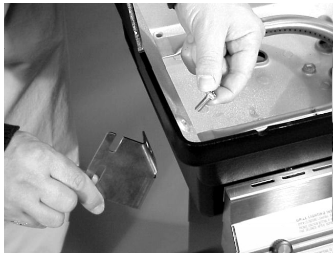
Figure 9 Installing Shelf Bracket
