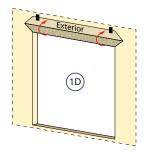
E. **Apply sill flashing tape #1.** Cut a piece of flashing tape 12" longer than the opening width. Apply at the bottom of the opening as shown (1E) so it overhangs 1" to the exterior.
