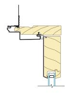
A. **Apply side flashing tape.** Cut two pieces of flashing tape 4" longer than the frame height of the door. Apply one piece 1/2" onto the frame cladding, over the nailing fin and onto the water resistive barrier. The tape should extend 2" above the top of the door and 2" below the bottom of the door. Press the tape down firmly while folding down the excess tape at the top and bottom of the door.
