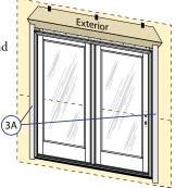
B. **Apply top flashing tape.** Cut a piece of flashing tape long enough to go across the top of the door and extend at least 1" past the side flashing tape on both sides. Apply the tape 1/2" onto the frame cladding, over the top nailing fin as shown. Fold the overlapping tape down, and press all tape down firmly.
