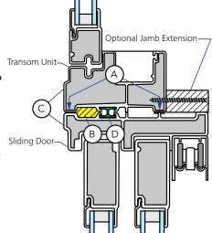
E. Apply sealant to the ends of the mullion joint. The bead of sealant should extend from the center of the mullion joint to the exterior of the unit, covering the foam plug.
