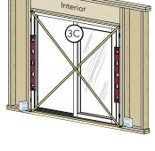
E. Install roller retainers. Position and secure the two roller retainers provided by drilling pilot holes through the pre-drilled holes into the sill support. Apply sealant to the holes and insert screws as specified below:
