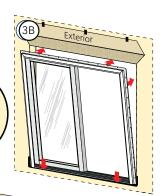
C. Plumb and square door. Insert shims, as necessary, between the door and the sides of the rough opening starting up 6" from the bottom of the door. Keep shims back 1/2" from interior face of window.
