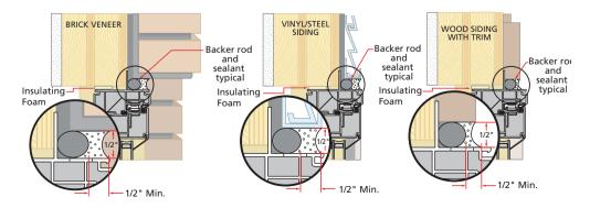
A. **Insert closed cell foam backer rod** into the space around the door approximately 1/2". This should provide at least a 1/2" clearance between the backer rod and the exterior face of the door.
