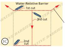
4th cut: Make a 6" cut up from each top corner at a 45° angle to allow the water resistive barrier to be lapped over the fin at the head of the door.
