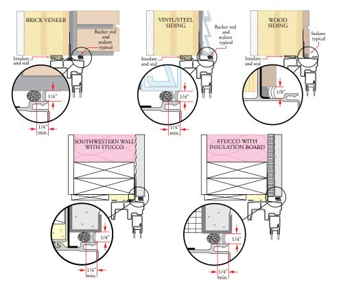
A. **Insert closed cell foam backer rod** into the space around the window as deep as it will go. This should provide at least a 1/4" clearance between the backer rod and the exterior face of the window.
