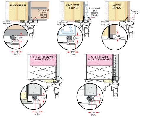
A. **Insert closed cell foam backer rod** into the space around the window as deep as it will go. This should provide at least a 1/4" clearance between the backer rod and the exterior face of the window.
