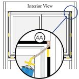
Note: It may be necessary to squeeze the end of the tube with pliers to be able to insert into the space between the window frame and the rough opening. DO NOT completely fill the space from the back of the fin to the interior face of the opening.
