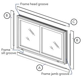
D. Seal the over-lapping fin joints with sealant.
