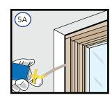
Note: It may be necessary to squeeze the end of the tube with pliers to be able to insert into the space between the window frame and the rough opening. DO NOT completely fill the space from the back of the backer rod to the interior face of the opening.
