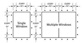
A. Casement: On the room side of the window, drill 1/8" diameter clearance holes through the head, jambs and sill of the frame. Space the holes a maximum of 6" from each end and a maximum of 16" on center.
