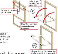
G. With the sash parallel to the floor, lift one side of the upper sash until the terminal is removed from the balance shoe. Continue to lift the sash up until the terminal is released from the opposite side of the sash and can be removed from the shoe. Lift the sash up and out of the window frame. Set the sash in a safe location.
