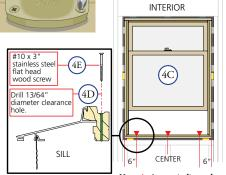
Note: Arrows indicate the placement of clearance holes.
