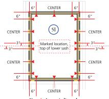
Note: Arrows indicate the placement of clearance holes.
