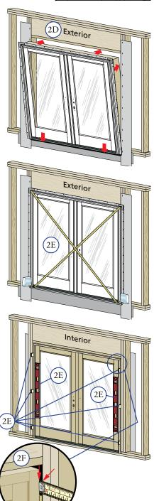
G. **Fasten the door to opening** by driving 2" galvanized roofing nails into each pre-punched hole in the nailing fin.
