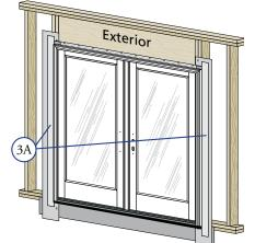
B. **Apply top flashing tape.** Cut a piece of flashing tape long enough to go across the top of the door and extend at least 1" past the side flashing tape on both sides. Apply the tape 1/2" up onto the frame cladding, over the top nailing fin as shown. Fold the overlapping tape down, and press all tape down firmly.
