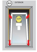
Note: Each existing window frame and wall depth will vary in different applications; therefore there is not a standard measurement for the overhang of the window frame to the exterior or for the distance from the interior face of the window to interior trim. When performing Steps 4B thru 4C, installing the frame screws, be sure to keep the distance consistent all around the window.
