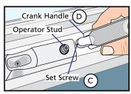
E. **Fold the crank** handle down and check alignment of knob with the pocket.
