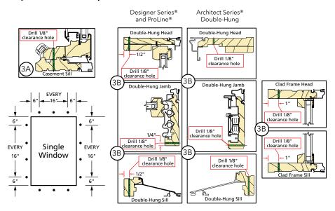
B. Double-Hung and Clad Frame: On the room side of the window, drill 1/8" diameter clearance holes through the frame at the locations shown. Space the holes a maximum of 6" from each end and a maximum of 16" on center.
