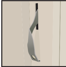
Construction Handle Tool may be used as a lock handle or crank handle.
