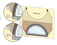
B. For Curve Top Windows: Several pieces of flashing tape will be needed to cover the top fin.
