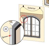
F. **Plumb and square window**. Place shims 1" from the bottom and top of the window between the window and the sides of the opening. Adjust the shims as required to plumb and square the window in the opening. If the frame height exceeds 53", place shims at the midpoint of the window sides.
