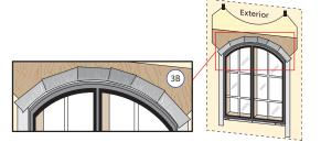
C. Apply top flashing tape to an angle top window 1/2" up onto the frame cladding, over the top fin onto the sheathing. On the short side of a trapezoid window, do not allow the side flashing tape to extend higher than what the top tape will cover. Fold the overlapping tape down, and press all tape down firmly.
