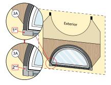
B. For Curve Top Windows: Several pieces of flashing tape will be needed to cover the top fin. Start taping from the sides of the window working toward the peak. To determine the length of cuts, hold the tape along the radius, and cut the
