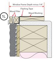
M. Install and level sill spacers. Place 1" wide x 1/4-3/8" thick spacers on the bottom of the window opening 1/2" from each side and 1/2" back from the interior surface of where the new window will rest. Spacers are also required below mullions and at screw anchor locations.
