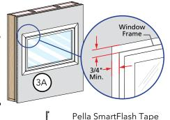
B. Apply Pella SmartFlash tape across the head of the window extending 6" down each jamb. Place the tape starting on the aluminum cladding and extending onto the wood frame.
