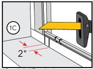
D. Use pliers to remove the 2" section(s) of frame.
