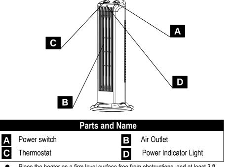
Place the heater on a firm level surface free from obstructions, and at least 3 ft. away from any wall and any other objects such as furniture, curtains, plants or combustible material.
