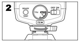
● PENTAX digital single lens reflex cameras can accept a shoe lock pin. When attaching the flash unit, turn the locking lever in the (FIX→) direction and lock the flash unit to the camera with the shoe lock pin. When releasing the flash unit, be sure to do so after turning the locking lever in the direction opposite to that indicated by (FIX→) and loosening the shoe lock pin. Otherwise, the hot shoe will be damaged.
