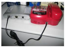
2. Connect Gateway to Internet: plug the RJ-45 Ethernet cable into the Ethernet Jack. Plug the other end of the cable into HUB.
