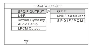
Precautions: In Audio Setup, SPDIF OUTPUT controls simulating output or optical output, and simulating audio output is prohibited where optical output exists.
