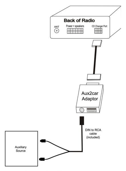
Connect Auxiliary source to female RCA input
