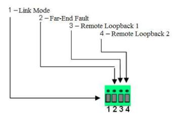
**Note:** All switch changes take effect immediately and will result in a link reset on both fiber ports.
