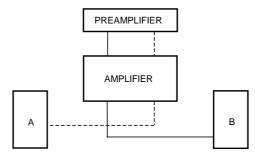
Change the loudspeaker leads from one loudspeaker to the other. If the fault remains in loudspeaker 'A', then loudspeaker 'A' is at fault, go no further.
