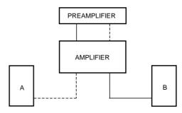
Change the loudspeaker leads completely from left channel to right and from right channel to left by now swapping them at the amplifier output. If the fault now appears in loudspeaker 'B', then that loudspeaker lead is at fault, go no further.
