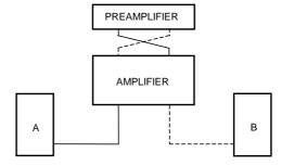
Change the input plugs on the rear of your amplifier, as follows: Change each input source in turn by swapping the plugs left to right and right to left. If the fault changes to loudspeaker 'B' on any one of the selected inputs, then that particular input source is possibly at fault. Move on to step 3b.
