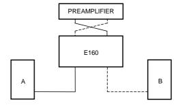
Change the input plugs on the rear of your amplifier, as follows: Change each input source in turn by swapping the plugs left to right and right to left. If the fault changes to loudspeaker 'B' on any one of the selected inputs, then that particular input source is possibly at fault. Move on to step 3b.
