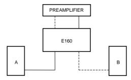
Change the interconnect leads completely from left channel to right and from right channel to left by now swapping them at the source component's output. If the fault stays in loudspeaker 'B', then the interconnect lead is at fault, go no further.
